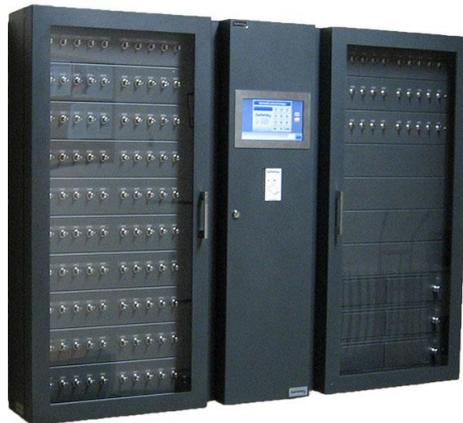
Apply the EKD card/student ID card to the reader, which is located under the touch screen. Select the keys you want to collect by pressing on the names of the keys and confirm with the "Enter" button. After selecting a key, the door will release and the LED indicating the location of the selected key will illuminate. Remove the key ring and close the door of the depository.
